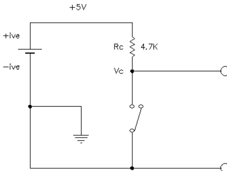
If a voltage is applied to the input through the 4.7K resistor, it causes a small current to flow through the base-emitter junction of the transistor. This causes the transistor to “turn on” and become like a closed switch. Using the principal of a series voltage divider the circuit would then look like the diagram below:
