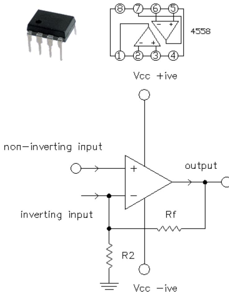
Because they have such high gain and wide frequency response, they are very useful with simple feedback circuits such as filters and so on. In this diagram the op-amp is being used with a "non-inverting" output, and the -ive input is being used for negative feedback. The formula for the gain with feedback is:
