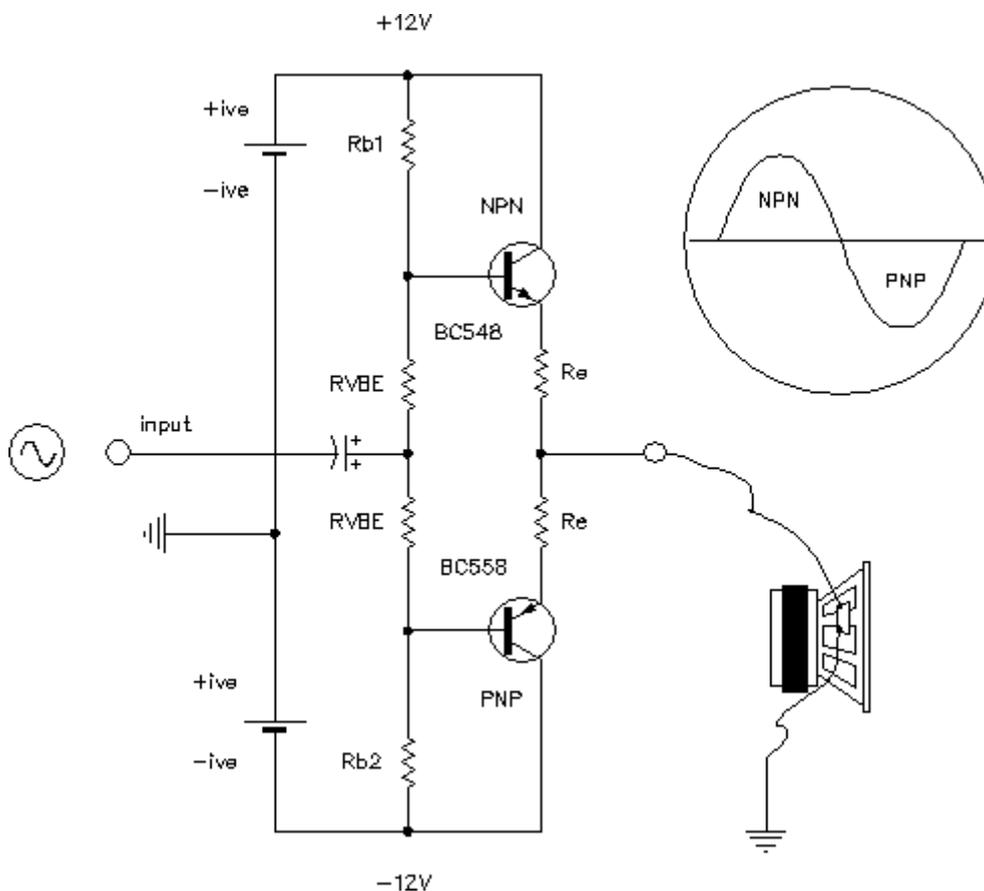
When the top (NPN) conducts, the bottom (PNP) is turned off & visa versa. The transistors complete the circuit by conducting the + & - DC supply's current through the loudspeaker, to earth and to the middle of the two batteries. Because the two batteries are earthed in the mid point of the + & - 12V, the two emitters of the transistors are at 0V with reference to earth. Most modern amplifiers use this system in one form or another.
