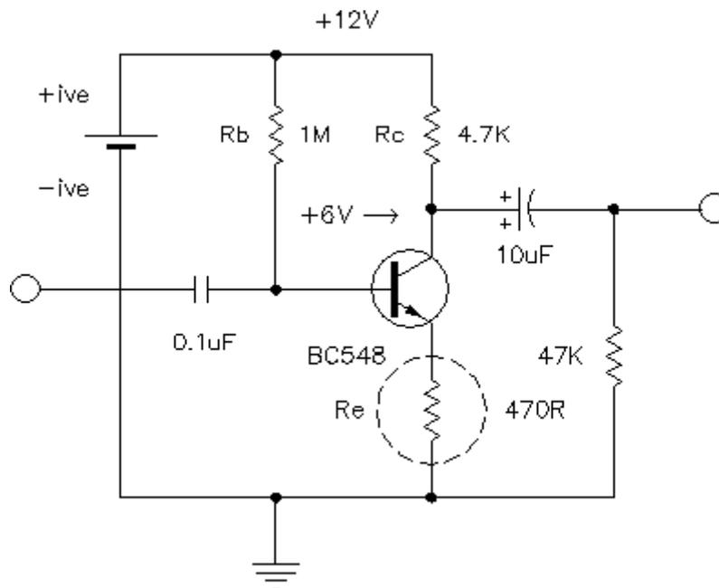
In this circuit we have included a resistor ( $R_e$ ) in the emitter to ground connection. This means that when the current flow increases in the transistor due to a positive signal, a voltage drop occurs across  $R_e$ , and this raises the voltage at the emitter causing the base-emitter voltage to **reduce**. It effectively **reduces the amplification** factor of the transistor. This is called ‘**negative feedback**’.
