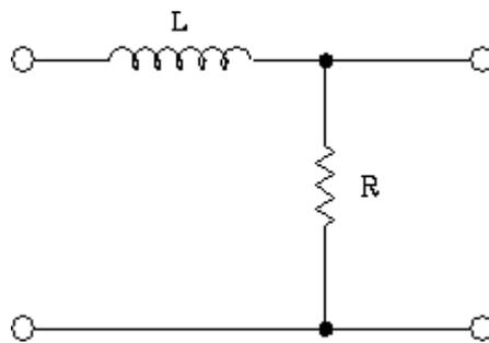
And the circuit above must be a \_\_\_\_\_ pass filter because \_\_\_\_\_ frequencies encounter a high resistance between the input and the output.
