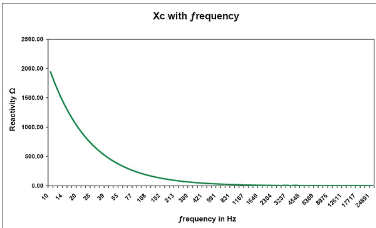
By re-arranging the formula for  $X_c$  we can predict the “turnover” frequency for any given combination of  $R$  &  $C$ . i.e. when the capacitive reactance of a cap is the same value as the series resistor, we can substitute  $X_c$  for  $R$ . E.g.
