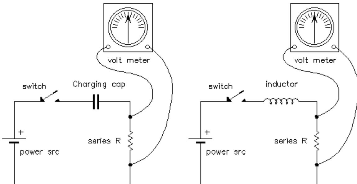
If we looked at the voltage over the 'series R' resistor in the 1<sup>st</sup> diagram, it would look like the diagram on the next page: the capacitor **accepts** the flow of current quickly at first, but slows exponentially, until there is no current flow.
