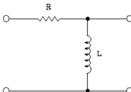
This circuit must be a \_\_\_\_\_ pass filter because \_\_\_\_\_ frequencies are bypassed to ground.
