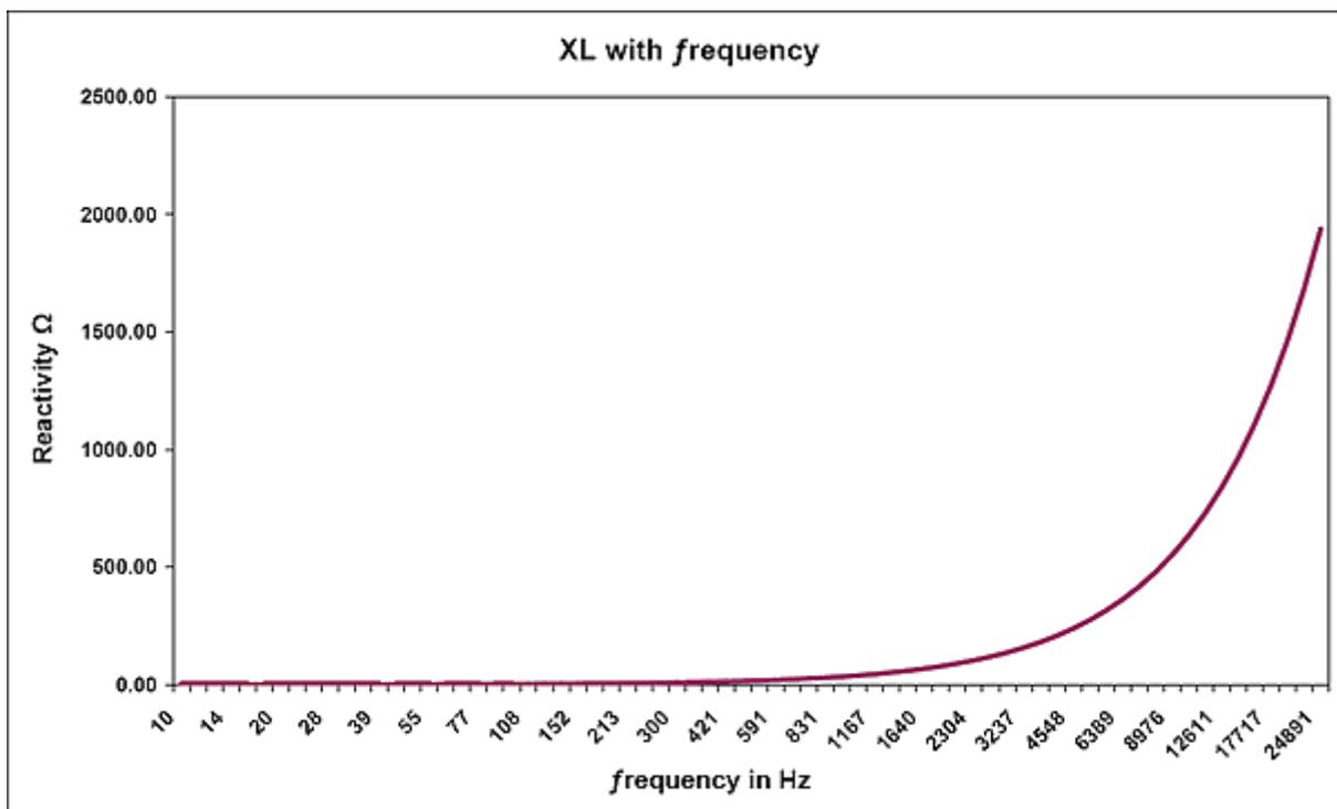
We can calculate the actual value of inductive reactance for any given inductor if we know its value and the frequency of the input sine wave.
