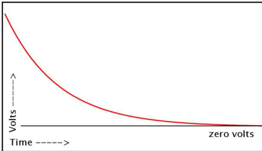
If we looked at the voltage over the 'series R' resistor in the 2<sup>nd</sup> diagram using an inductor, it would look like this: the inductor **resists** the flow of current, but this effect decreases exponentially and eventually the DC flows through unhindered. **Note that in both cases we are measuring the voltage changes over the series resistor.**
