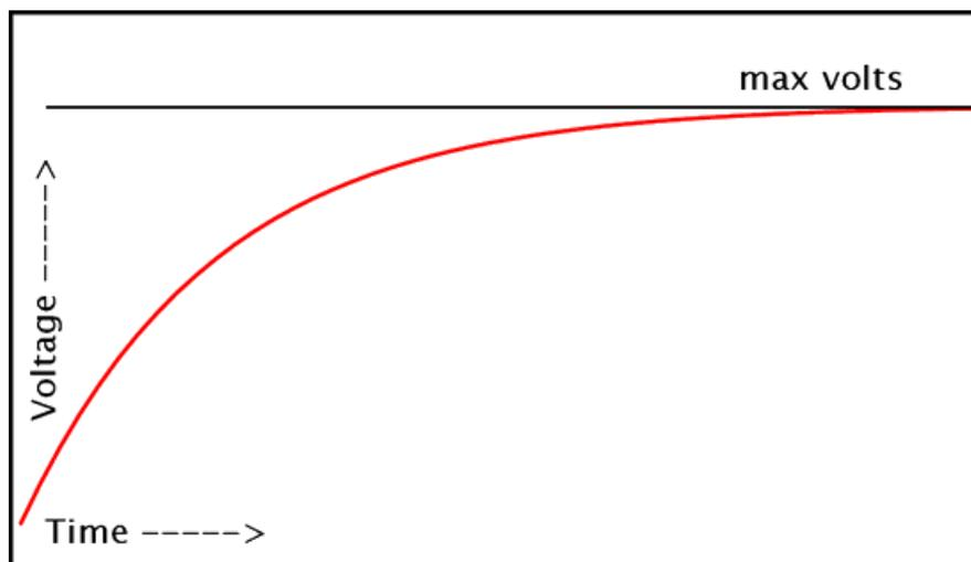
We still use the Universal Time Curves to describe the operation of a series Inductance Resistance circuit but this time on the charging cycle the rising curve is the circuit current. A series LR circuit also takes 5 time constants to reach it fully charged condition.
