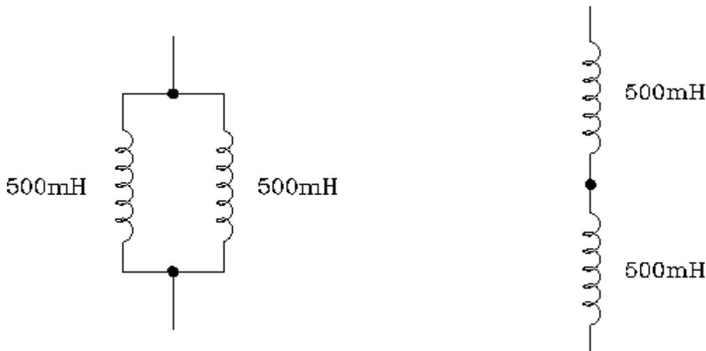
It is not a very common practice to connect inductors in parallel or series for that matter and if they are they are usually the same values so working out the total inductance is a relatively simple exercise.
