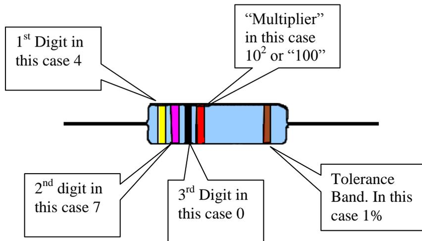
So this resistor is a  $470 \times 10^2 (100) = 47,000\Omega = 47K\Omega @ 1\%$  tolerance.
