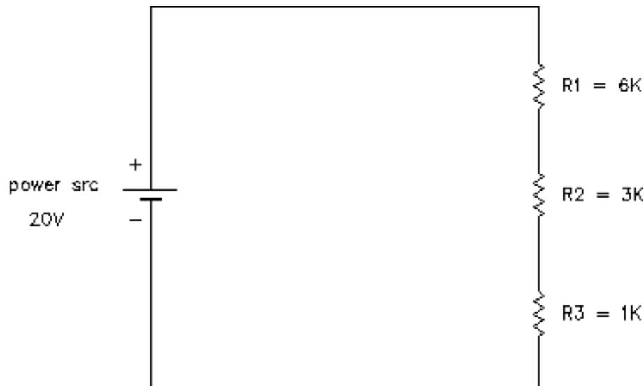
We can assume that the total resistance of the series resistances is equal to the sum of the resistors. Therefore  $R_{\text{total}} = R1 + R2 + R3$  which = 10K (10,000 $\Omega$ )
