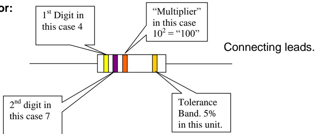
So this resistor is  $4700\Omega$  5% or  $4.7K\Omega$  5% Actual size is about 10mm x 2mm. ie.
